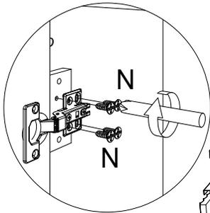
Assemble these four holes first, adjust the door and ensure it is level, then tighten all screws.
